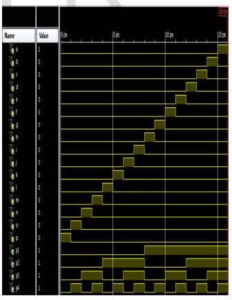
Figure15: Waveforms of 16:4 Reversible Encoder.
