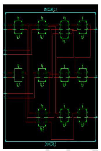
Figure 12: RTL view of 8:3 Reversible Encoder.
