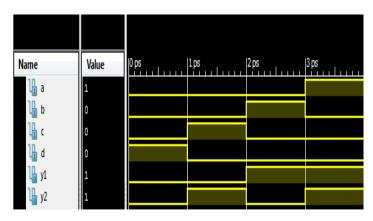
Figure 11: Waveforms of 4:2 Reversible Encoder.
