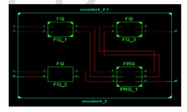
Figure 10: RTL view of 4:2 Reversible Encoder.
