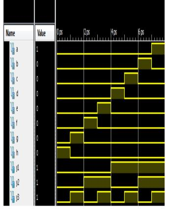
Figure 13: Waveforms of 8:3 reversible Encoder.
